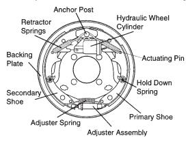
Figure 62. Hydraulic Brake Components
